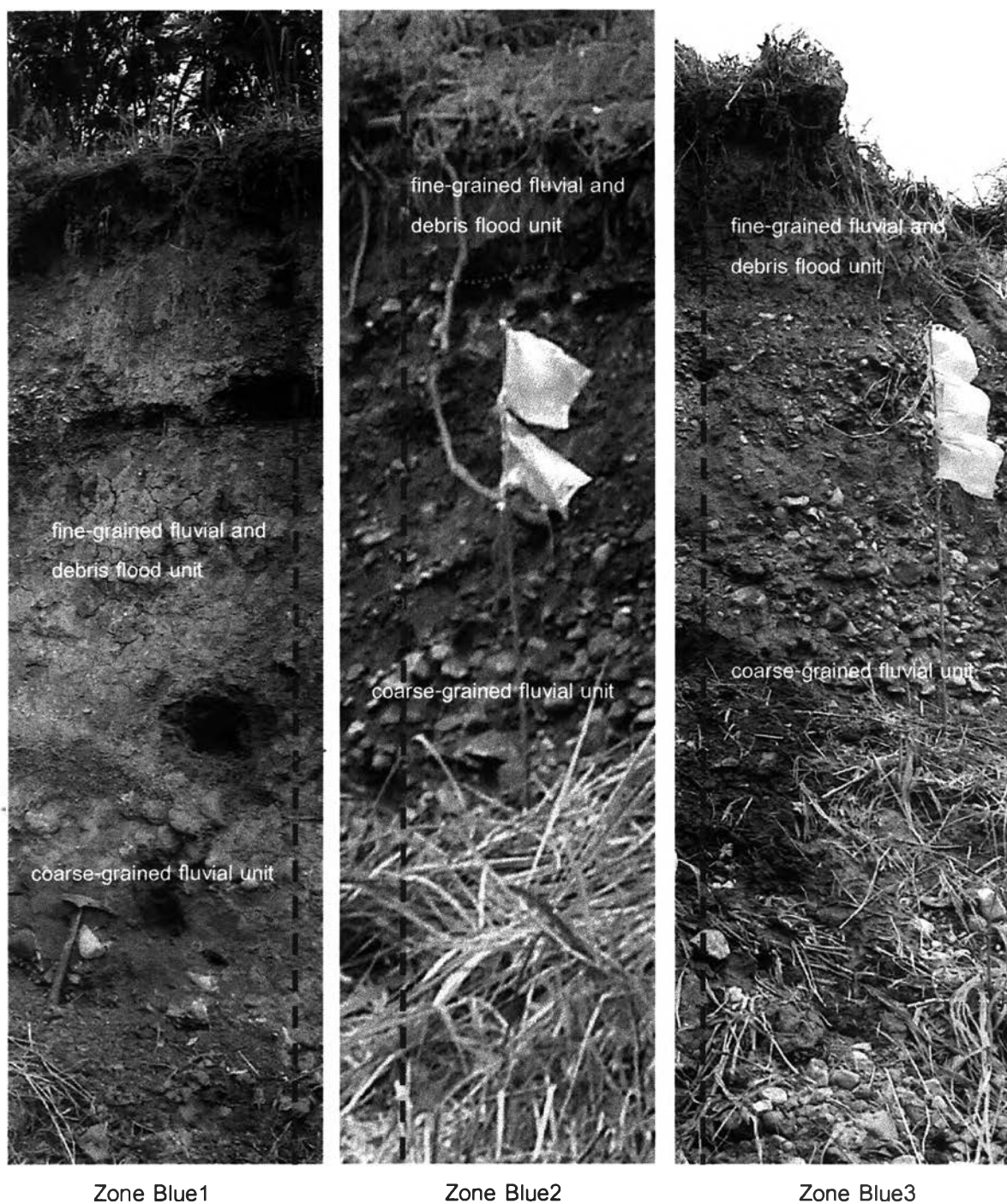
Figure 6-15 Photographs illustrating detailed sedimentary and stratigraphic characteristics in vertical succession of the fine-grained fluvial and debris flood unit that overlay with the sharp contact manner on top of the coarse-grained fluvial unit at the zones Blue1, Blue2 and Blue3.
