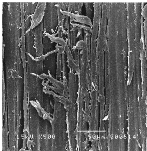
b. Wood treated with xylanase 0.05 u/ml at 32°C for 30 min, then treated with 10% H 2 O 2 and laccase 0.05 u/ml at 60°C for 4 hours
