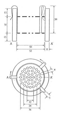
Figure 2. The apparatus for the disintegration of suppositories.
