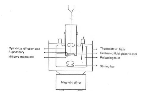
Figure 3. Cross-sectional diagram of the *in vitro* release and diffusion rate apparatus.
