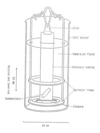
Figure 4. Diagram of the apparatus used in the modified dialysis membrane method.
