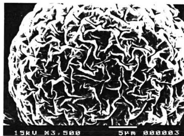
Figure 4.4 SEM photographs of the surface of poly(2-EHA-co-EGDMA) with various ratios of heptane:toluene, a) 3.5:3.5, b) 4.5:2.5, c) 5.5:1.5, d)7.0:0.
