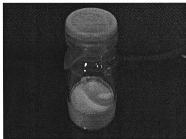
Figure 25 Freeze dried pralidoxime chloride annealed before the predetermined freezing temperature
