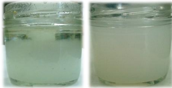
Figure B1 Characteristic of gelled electrolyte; a) the sedimentation of gelled electrolyte, b) gel characteristic of gelled electrolyte.
