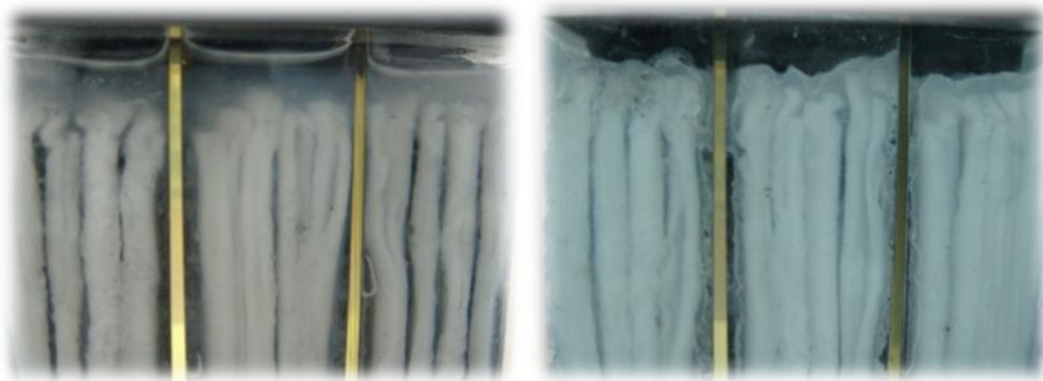
Figure B2 Characteristic of gelled electrolyte in VRLA battery; a) the sedimentation of gelled electrolyte, b) gel VRLA battery
