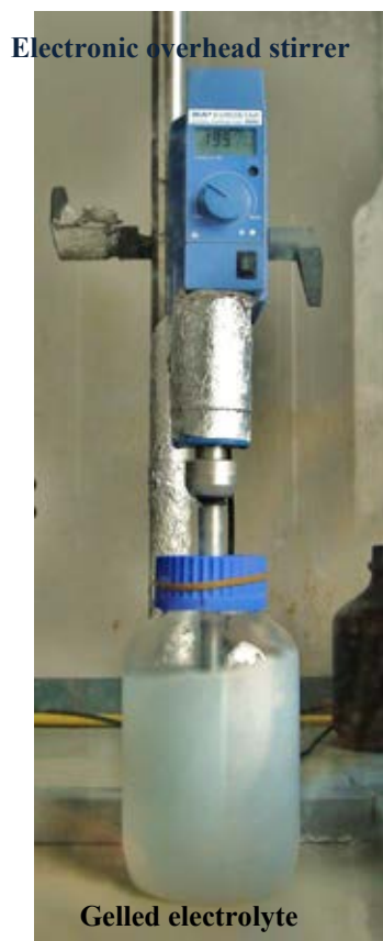
Figure 3.2 The setting of instruments for the gelled electrolyte preparation for industrial scale.
