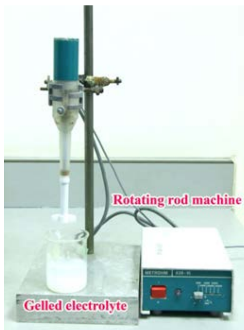
Figure 3.1 The setting of instruments for the gelled electrolyte preparation for lab scale.
