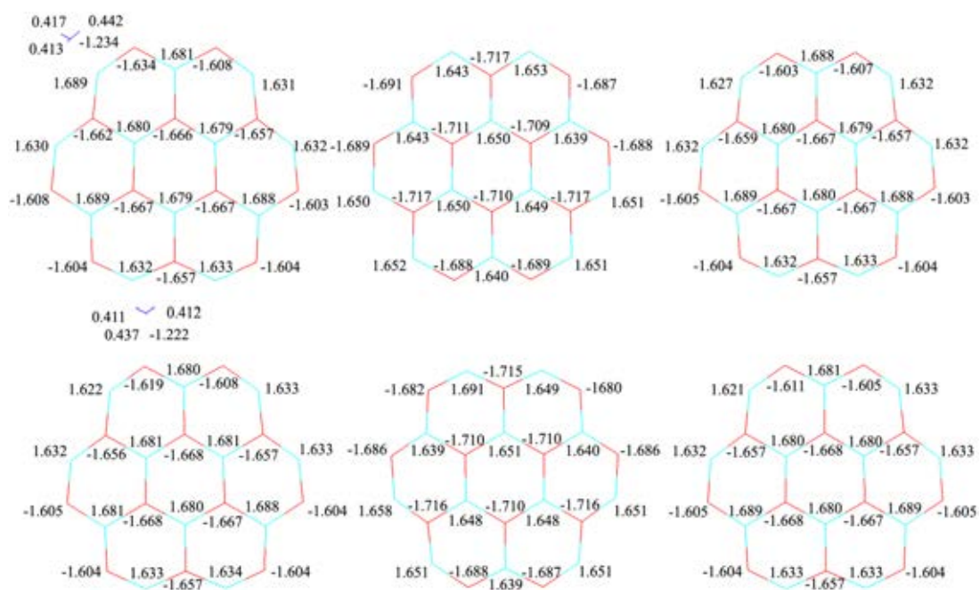
Figure A-6 NBO charges ammonia adsorption on (CNL-ZnONS') 3 (top) NH 3 / CNL-ZnONS' (1), (middle) NH 3 / CNL-ZnONS' (2) and (bottom) NH 3 / CNL-ZnONS' (3).
