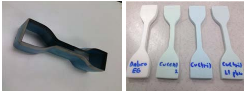
Figure 3.3 Dumbbell die C cutter following ASTM D412 and FPUR foams
