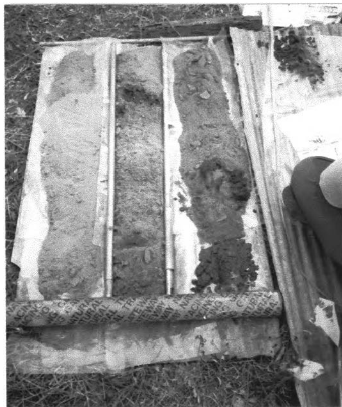
Figure 4.28 Sample from hand auger is mostly a very poorly sorted sandy silt layer and contains small amount of mica flakes and plant remains. (grid reference 038043)
