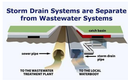
Figure 18 Storm drain system [37]
