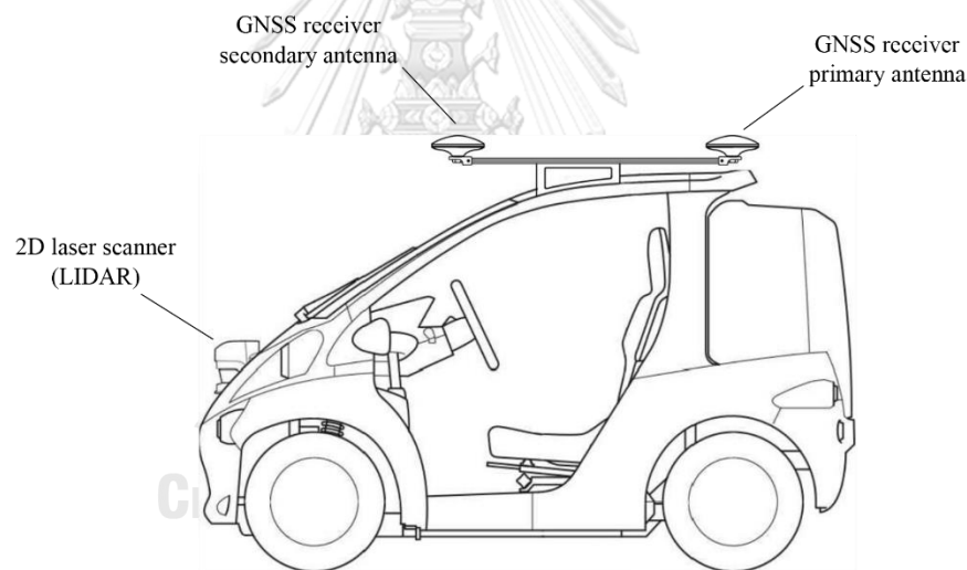
Figure 53 Test vehicle with the 2D laser scanner and the GNSS receiver installed
