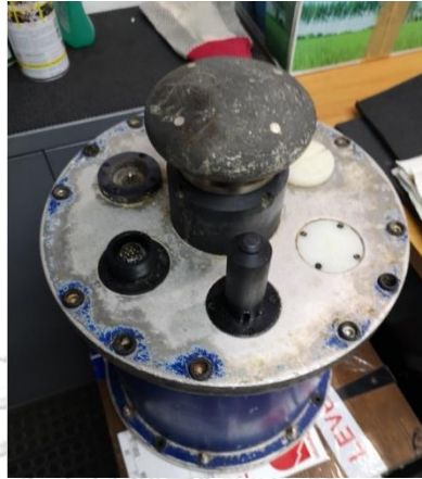
Figure 3 Device for wave magnitude and direction measurement
