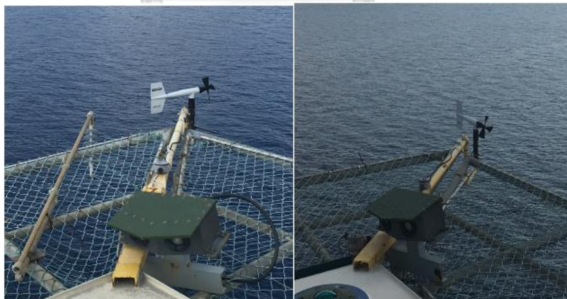
Figure 4 Anemometers located at NE (E1) and SW (E2) of living quarter
