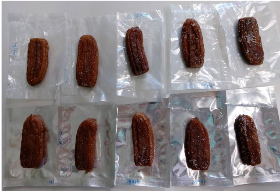
Figure 4.10 Sugar crystallization of dried banana which stored in both PB2 (above) and commercial (below) films at storage time 41, 54, 72, 84 and 112 days (from left to right)
