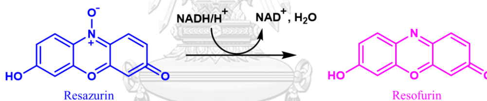
Figure 2.1: Reduction of resazurin to produce resofurin
