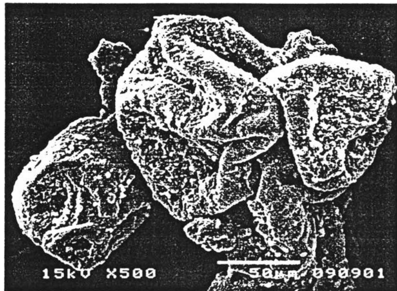
Figure 32 Scanning electron micrograph of BSA-TC walled D-panthenol microcapsules by using 20% w/v BSA and 16.6% w/v D-panthenol loading formulation D6.
