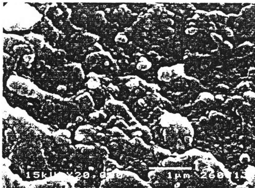
Figure 23 Surface morphology of BSA-TC walled D-panthenol microcapsules by using 13.3%w/v BSA and 10%w/v D-panthenol loading formulation D1. Magnification x 20000
