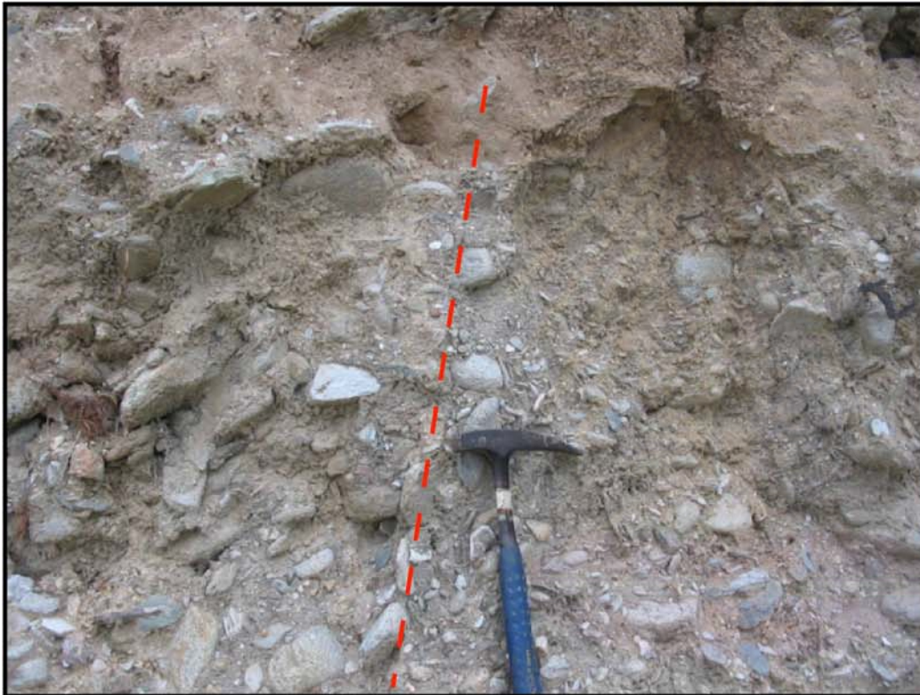
Figure 4.5b) Rolltating of gravel gains in semiconsolidated outcrop indicated faulting in young sediment.
