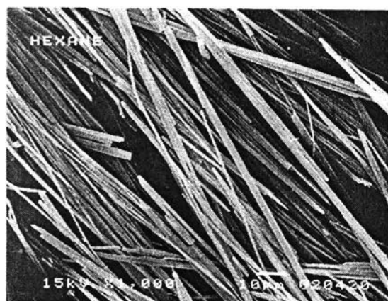
Figure 17: SEM (1000x) of VPU crystal recrystallized from hexane by method I
