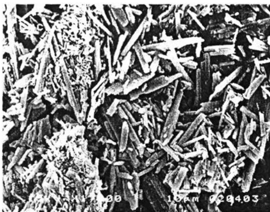
Figure 21: SEM (1000x) of crystal recrystallized from chloroform by method I
