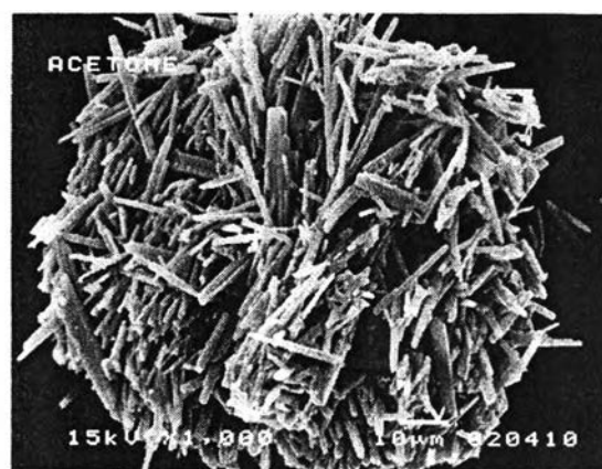
Figure 20: SEM (1000x) of VPU crystal recrystallized from acetone by method I
