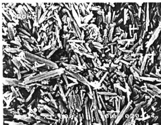
Figure 27: SEM (1000x) of VPU crystal recrystallized from methanol by method I
