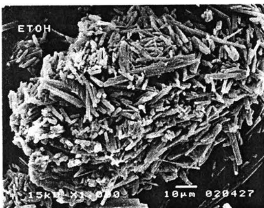
Figure 25: SEM (1000x) of VPU crystal recrystallized from ethanol by method I
