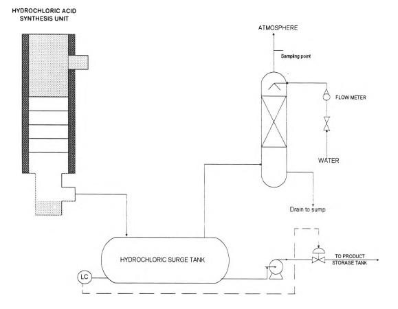
Figure 4.1 Scheme of the experiment on the existing packed absorber in plant site
