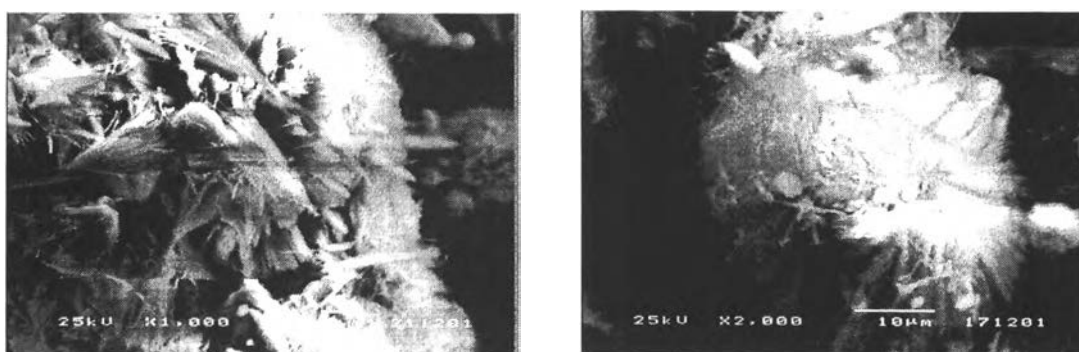
Fig. 2. SEM images of Pt/VPI-5 catalyst.
