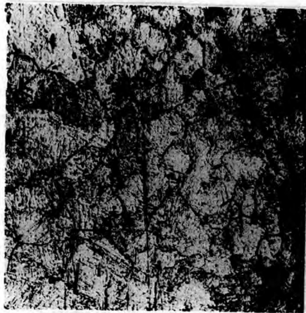
Figure 4.7 (b) Rolled 40% in recrystallization (100x)
