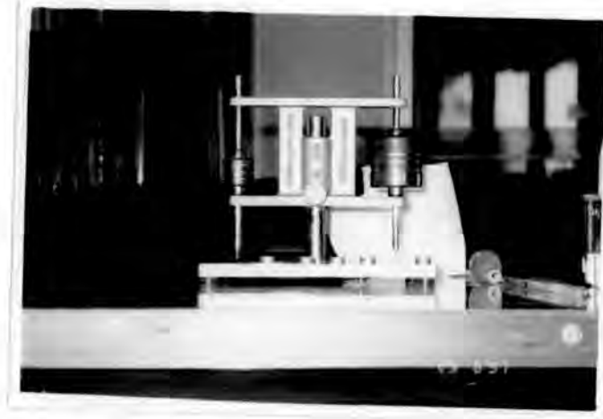
Fig. 3.13 Setting time testing instrument (Gillmore)
