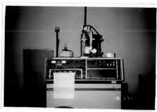
Fig. 3.5 Philips diffractometer, PW 1730/70
