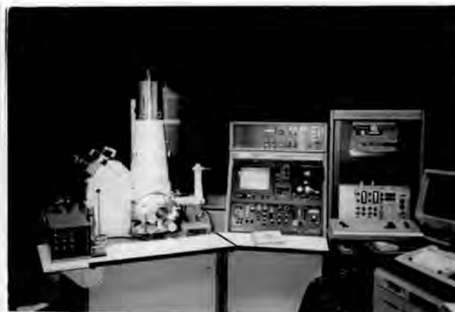
Fig.3.6 Scanning electron microscope (JSM T 220A, supplied by JEOL)
