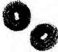
(a) 53 mm overall diameter particles with 20 mm diameter torus
