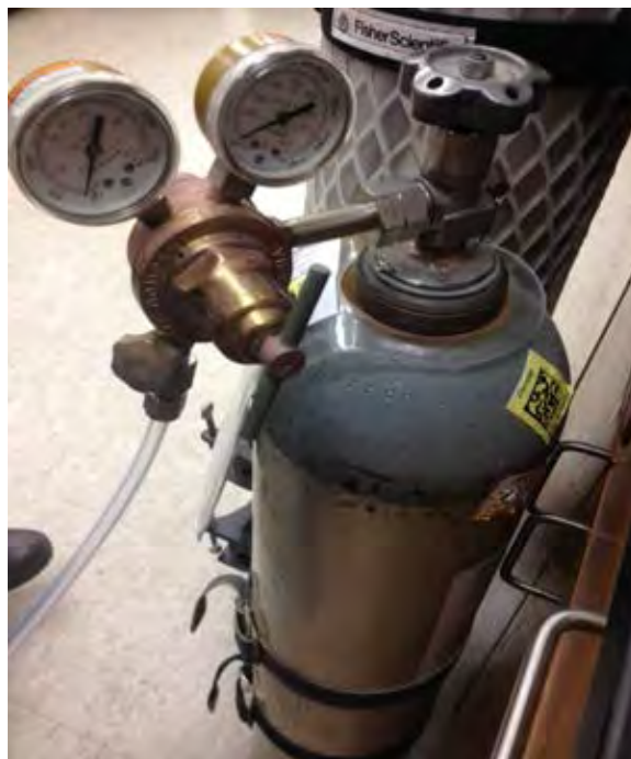
Figure 3.8 10 ppmv BTEX gas mixture for the experiment
