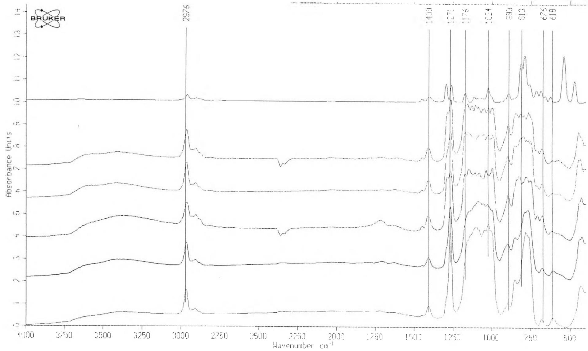
pure liquid 2-Cl silane KBr liquid cell
