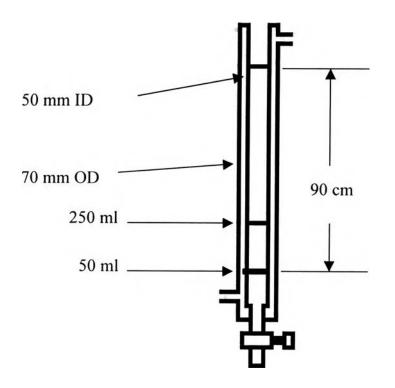
Figure 3.2 Foam receiver for the Ross-Miles test.
