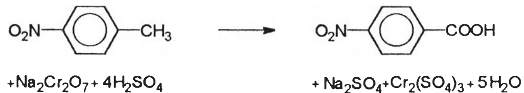
Figure 78. The chemical reaction of p -nitrotoluene with sodium dichromate in the acidic solution.
