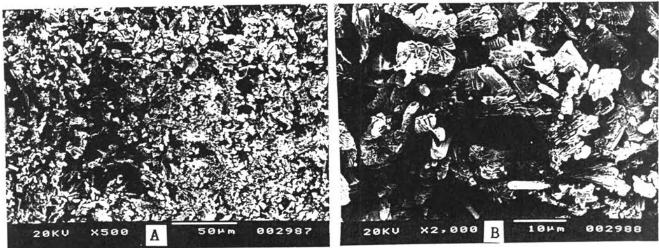
Figure 62 Photomicrographs of Spray-Dried Matrices after Release Testing (Cross Section) Key ( A x 500 , B x 2,000 )
