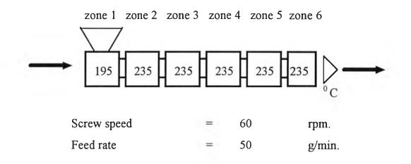
The extrudate was cooled in the water (~  $25 \circ$  C) and cut into pellet form by a Planetrol 075D2 pelletizer. The sample from each pass was collected for testing. The processed HDPE product was taken back into the hopper for the next pass with the same condition. The extruder was purged sufficiently to make sure that good material for each pass was attained.
