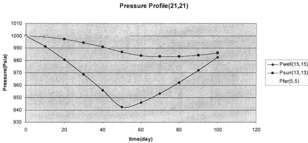
Figure 4.44 The pressure Profile of a 21, 21 grid reservoir.
