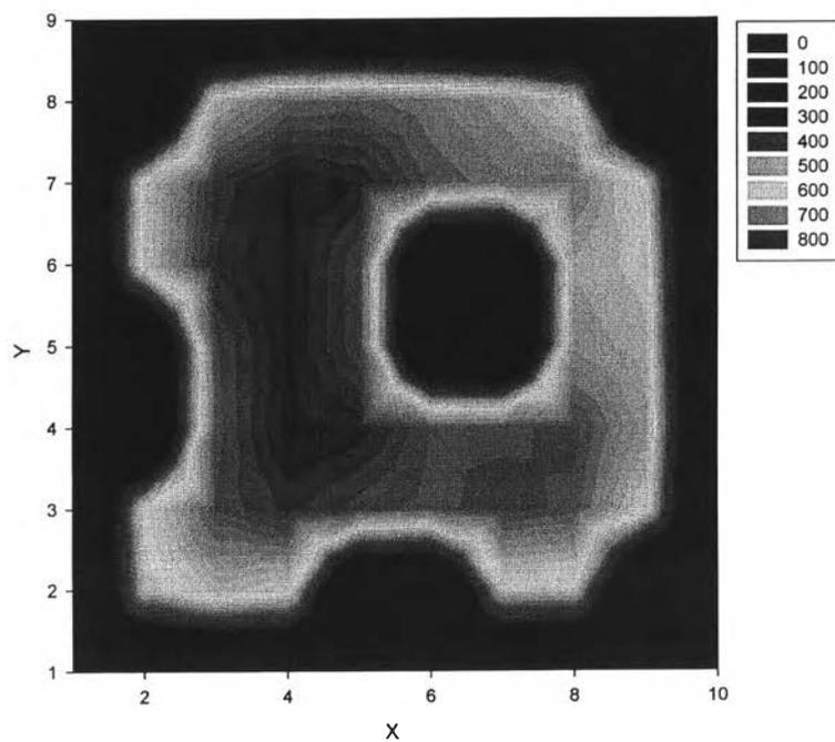
**Figure 4.24** Cross sectional view of pressure profile at T = 10 days.
