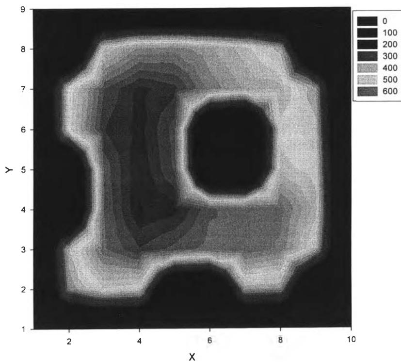
Figure 4.26 Cross sectional view of pressure profile at T = 100 days.
