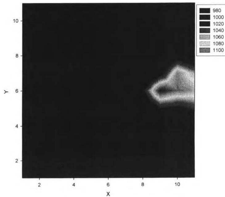
**Figure 4.14** Cross sectional view of pressure profile at T = 10 days.
