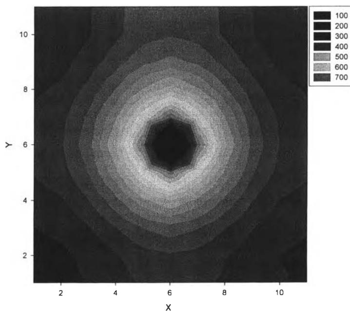
**Figure 4.3** Cross sectional view of pressure profile at  $t = 20$  second.
