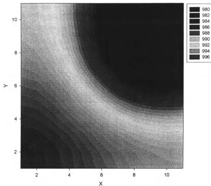
**Figure 4.6** Cross sectional view of pressure profile at t = 10 second.
