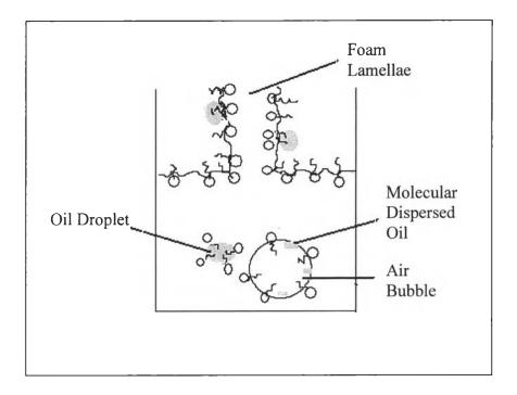
**Figure 1.1** Schematic diagram of froth flotation removal of oil from water (Wungrattanasopon, 1995).
