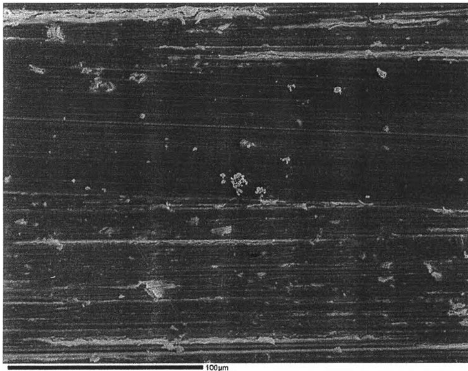
Figure 4.11 Deposits on the bottom coupon, Run2 at 500 magnification.
