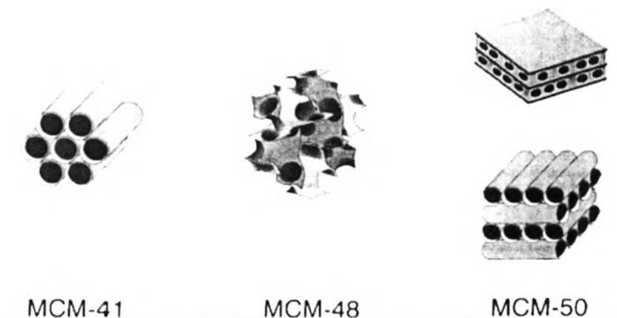
Figure 2.3 Structures for M41S mesoporous materials (Carreon et al. 2005).
