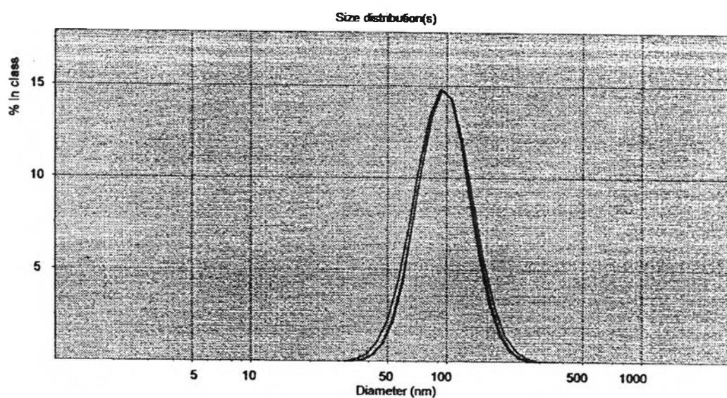
**Figure D11 : Particle size distribution of EA21/MAA14/E0.5/CM2.76/Tx10 latex**
