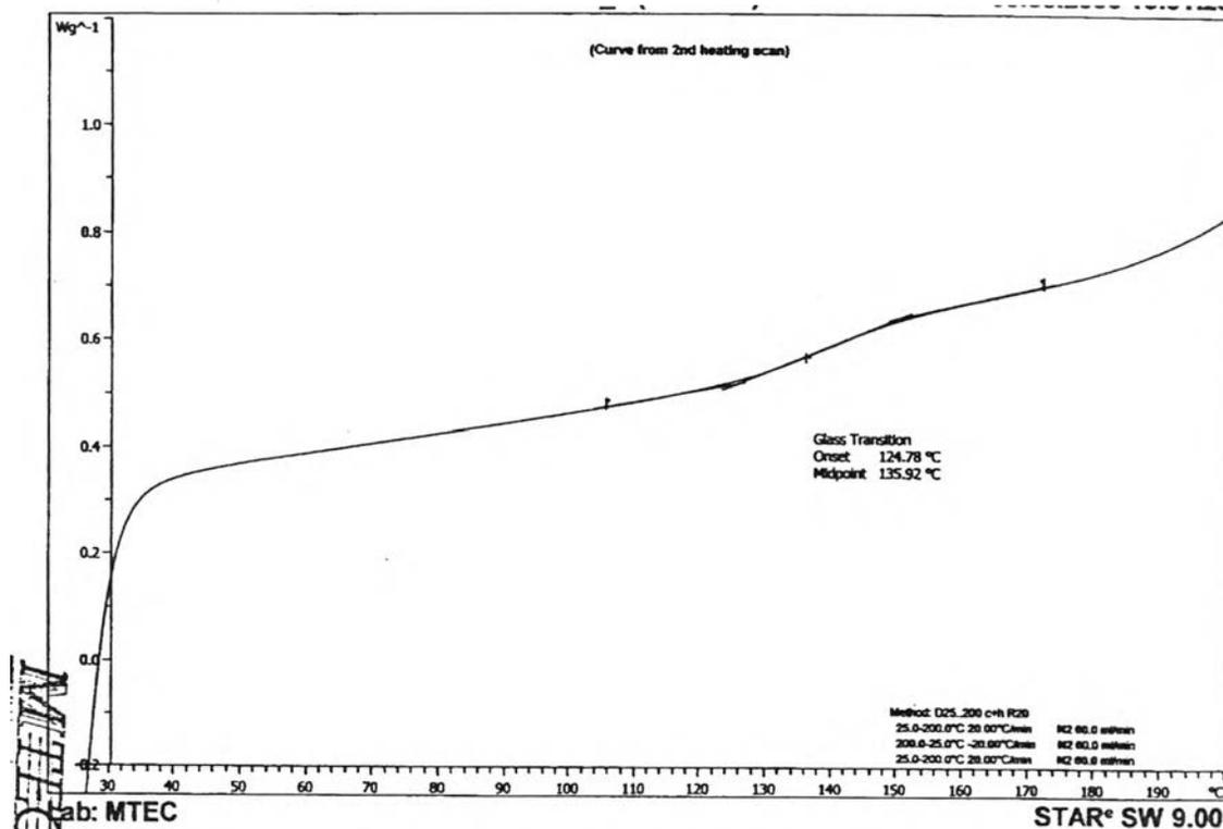
Figure C7 : Glass transition temperature ( $T_g$ ) of EA21/MAA14/E0.5/CM2.76
