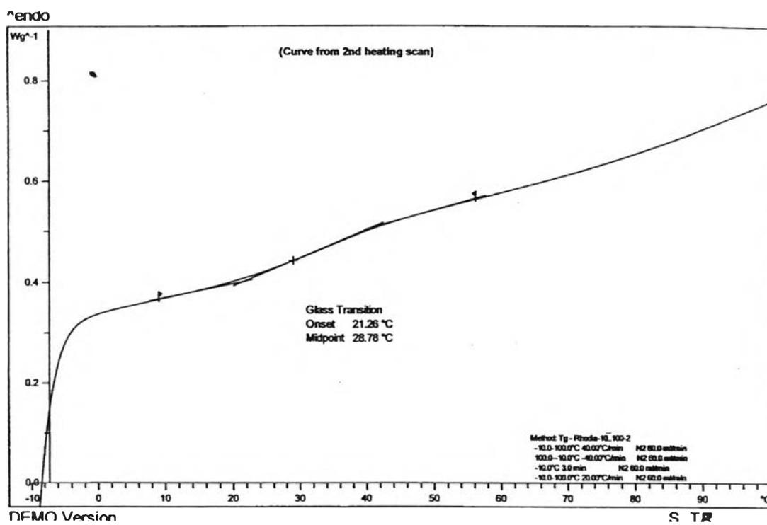
**Figure C9 : Glass transition temperature ( $T_g$ ) of EA21/MAA14/E0.5/CM2.76/Tx5**
