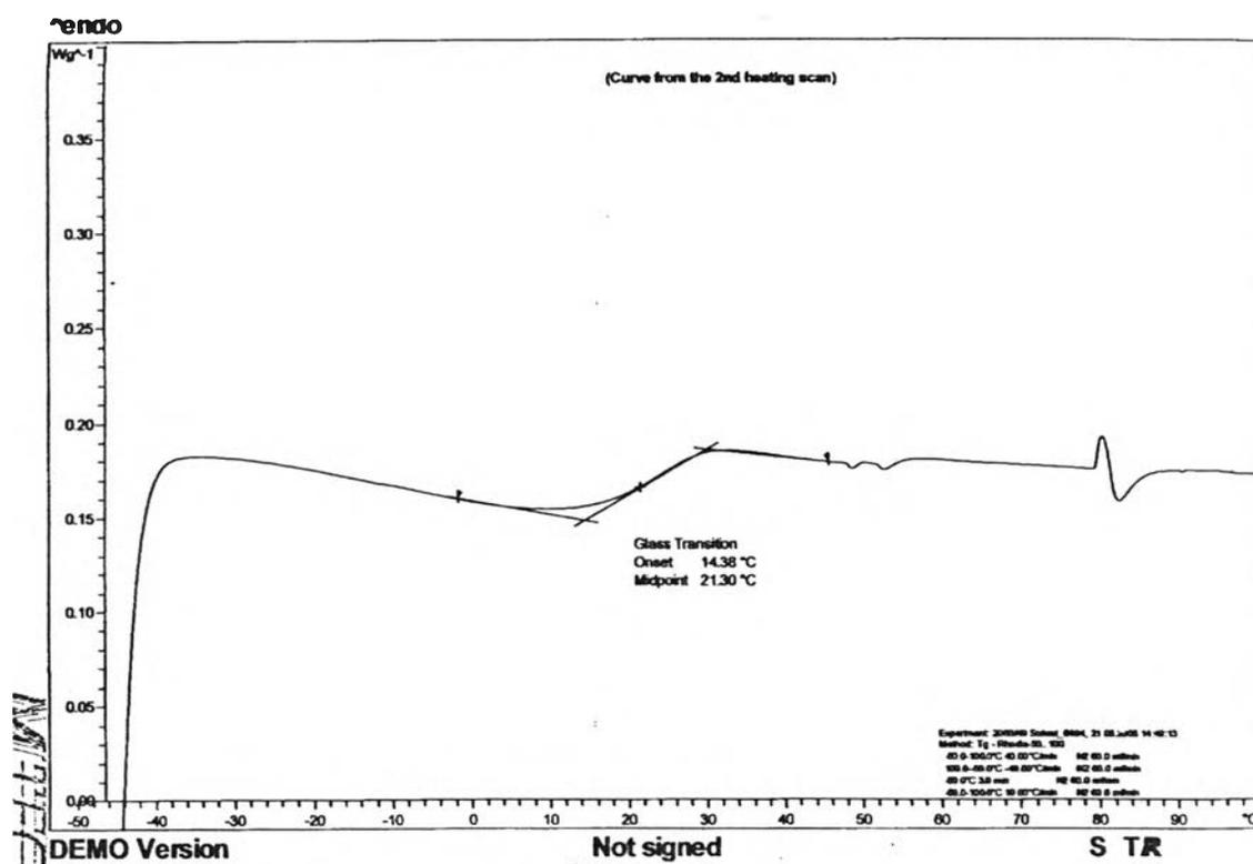
**Figure C4 : Glass transition temperature ( $T_g$ ) of EA21/MAA14/E0.5**
