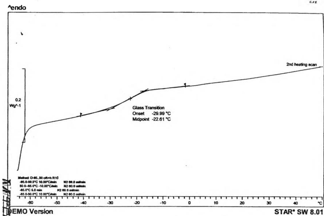
**Figure C13 : Glass transition temperature ( $T_g$ ) of EA21/MAA14/E0.5/CM2.76/Tx25**
