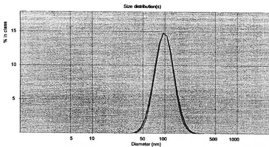
**Figure D12 : Particle size distribution of EA21/MAA14/E0.5/CM2.76/Tx15 latex**
