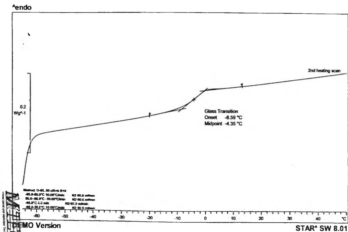
**Figure C12 : Glass transition temperature ( $T_g$ ) of EA21/MAA14/E0.5/CM2.76/Tx20**
