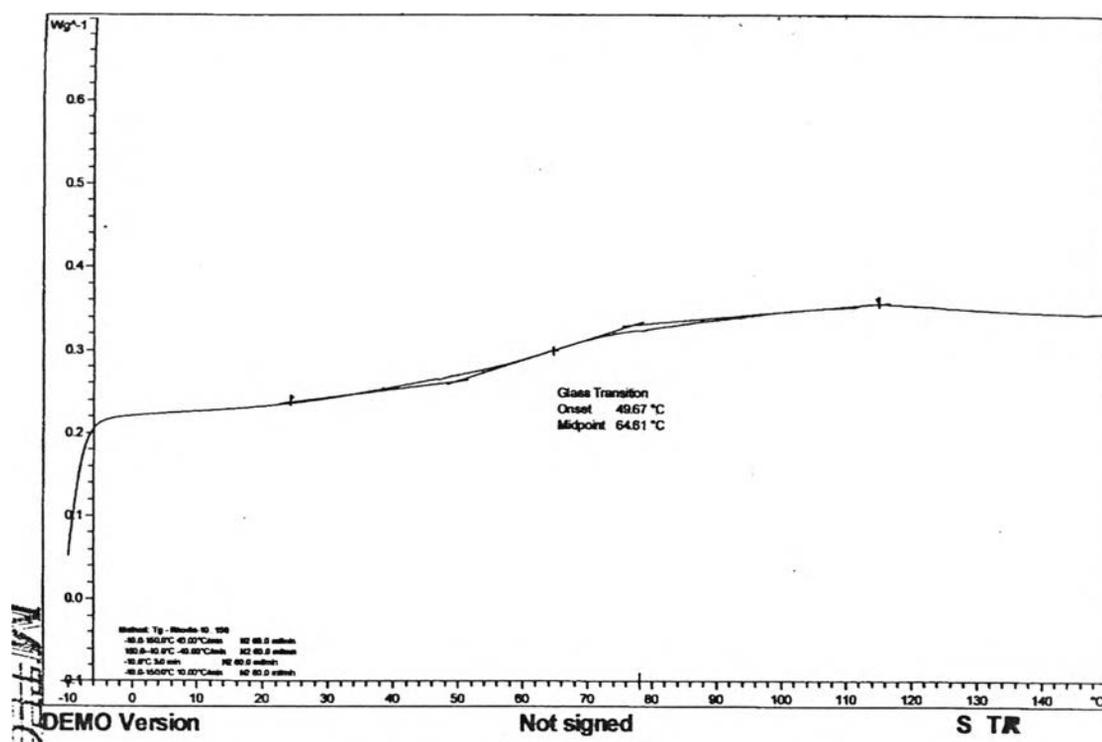
**Figure C6 : Glass transition temperature ( $T_g$ ) of EA13/MAA22/E0.5**
