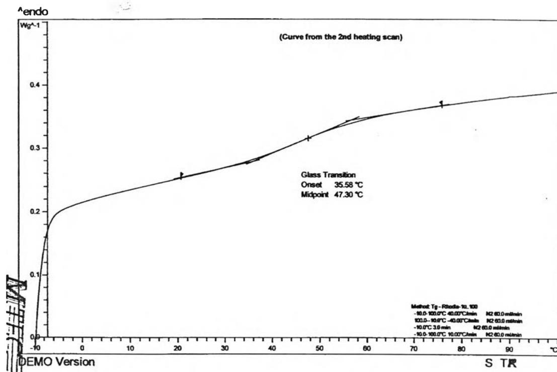
**Figure C5 : Glass transition temperature ( $T_g$ ) of EA18/MAA17/E0.5**
