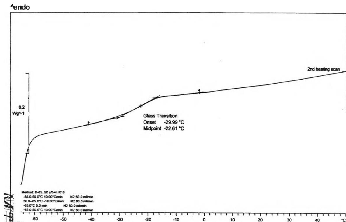
**Figure C2** : Glass transition temperature ( $T_g$ ) of EA35/E0.5
