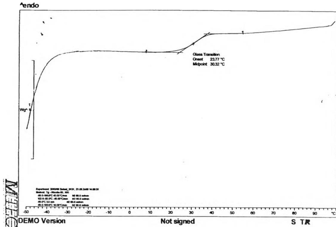
**Figure C10 : Glass transition temperature ( $T_g$ ) of EA21/MAA14/E0.5/CM2.76/Tx10**
