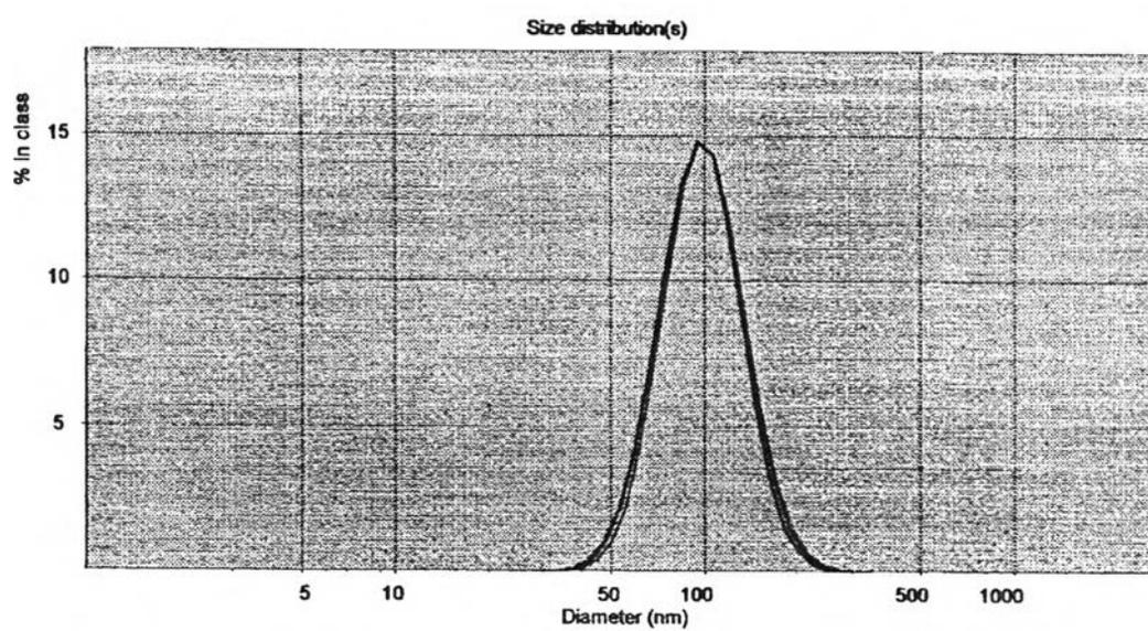
**Figure D13 : Particle size distribution of EA21/MAA14/E0.5/CM2.76/Tx20 latex**
