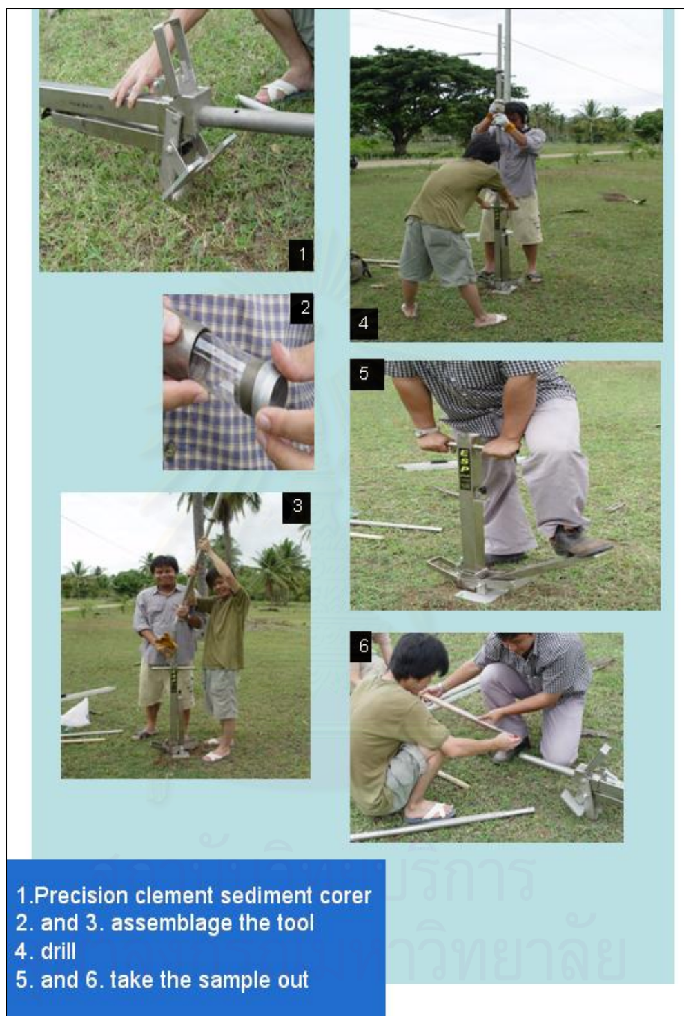
Figure 1.9 Taking sediment samples by using Precision clement sediment corer (ESP Plus).
