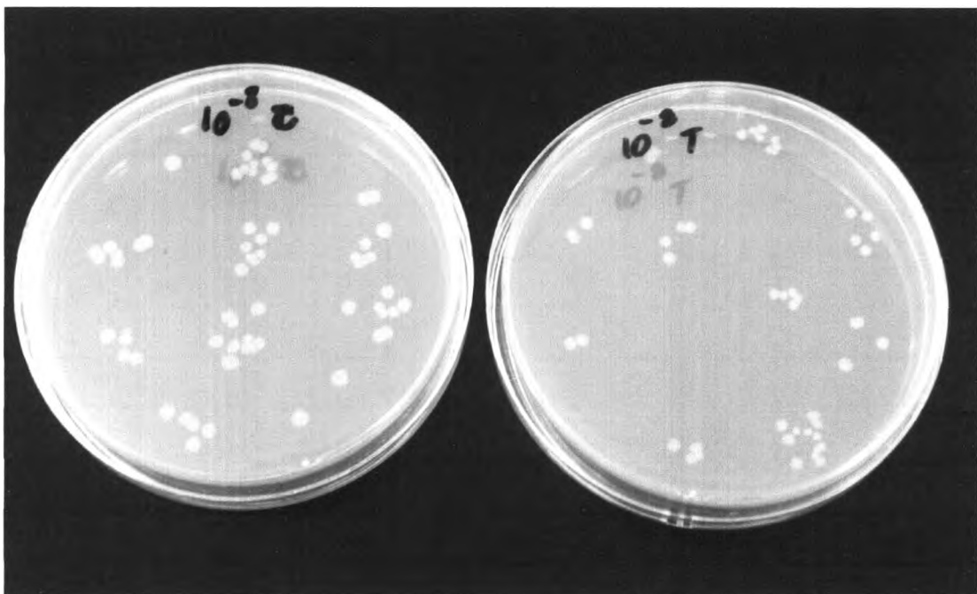
Figure 6.4 Agar plates of PP/OBEN-Cu20 nanocomposite films showing the numbers of E.coli colonies after incubated for 24 hours. The left agar plate was the control culture sample and the right plate was the PP/OBEN-Cu20 culture sample.
