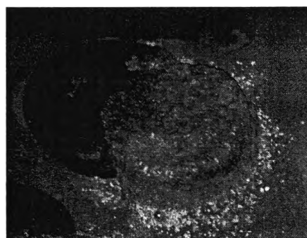
No.4, Limestone/ \text{Al}_2\text{O}_3+\text{SiO}_2 = 0.75 Complete Separation
