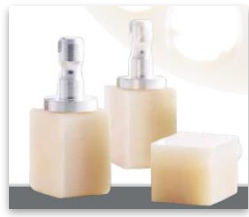
Shofu Block HC, VITA ENAMIC, Katana AVENCIA and Experimental material were cut into 4x4x1 mm 3
