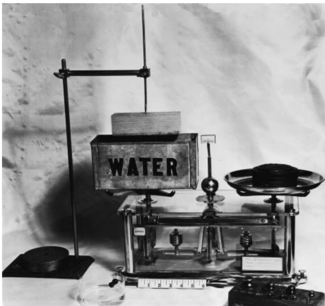
FIG. 39 Specific Gravity and Shrinkage-in-Volume Test Set-Up
