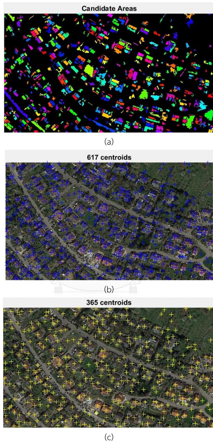
Figure 9 (a) Candidate areas, (b) Centroids of candidate areas before grouping the adjacency areas, and (c) Centroids of candidate areas after grouping the adjacency areas of the tested image T3.
