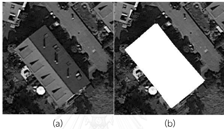
Figure 27 The sub-image of centroid number 156. (a) Original sub-image (b) Detected building resulted from the proposed line scanning.
