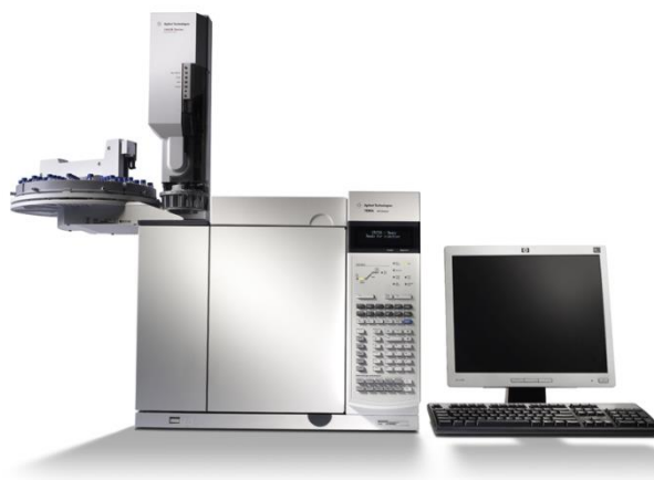
Figure 3.5 Agilent 7890A gas chromatograph for reaction product analysis.
