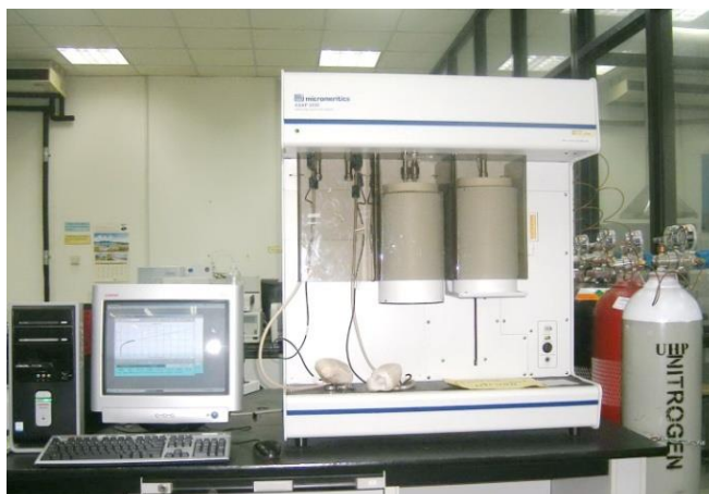
Figure 3.11 Micromeritics ASAP 2020 surface area and porosity analyzer.
