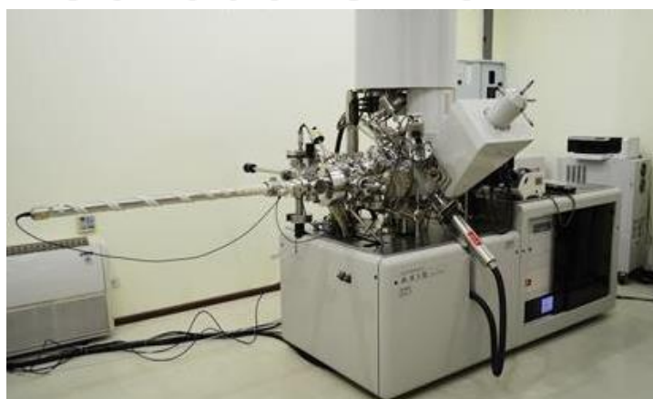
Figure 3.9 Kratos Axis Ultra DLD X-ray photoelectron spectrometer.
