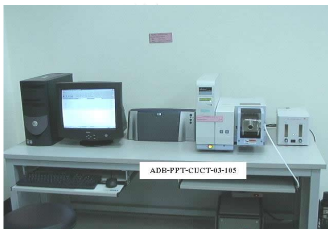
Figure 3.10 Perkin Elmer Pyris Diamond thermogravimetric/differential thermal analyzer.
