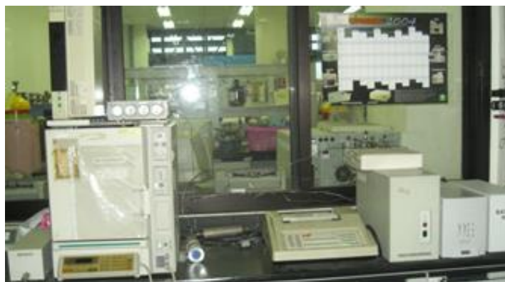
Figure 3.6 Shimadzu 14B gas chromatograph for reaction product analysis.
