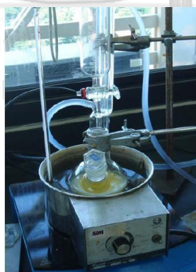
Figure 3.3 Experimental setup for the transesterification of RBD palm oil with methanol under batch conditions.
