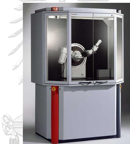
Figure 3.7 Bruker D8 Discover X-ray diffractometer.
