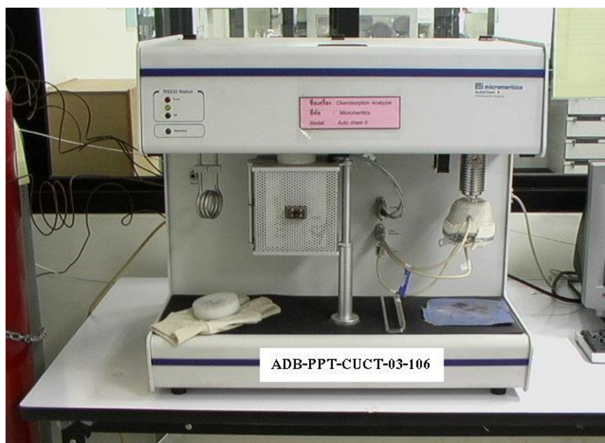
Figure 3.14 Micromeritics AutoChemII 2920 Chemisorption analyzer.
