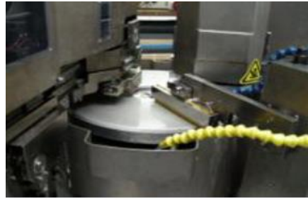
Figure 2.4 The lapping machine in the final lapping process [14]
