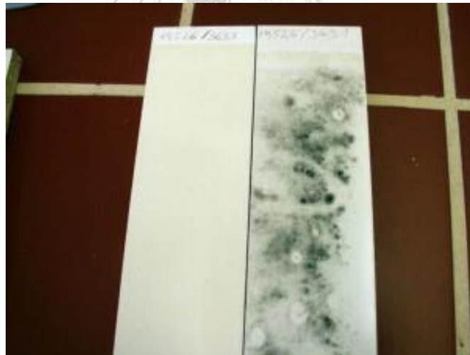
Figure 2.6 Antidust effect in case of surfaces with imidazolium salt on the left side and the reference surface without antistatic agent on the right side [12]
