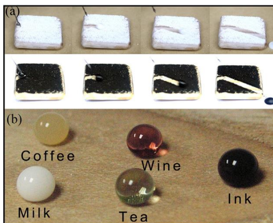
Figure 2.9 (a) The self-cleaning process and (b) Photograph of common household liquids on the SW1, respectively
