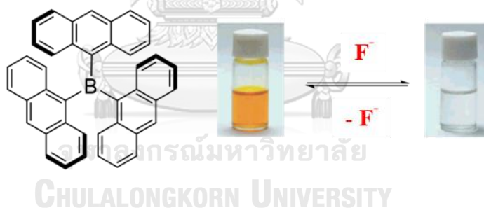
Figure 1.4 Colorimetric change of tris(9-anthryl)borane upon addition of F^- in THF.
