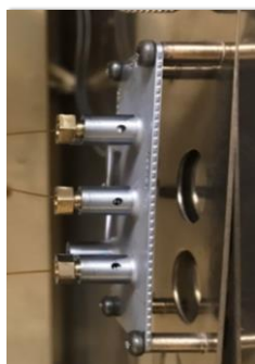
Figure 4. A three-port solenoid valve of DS.
