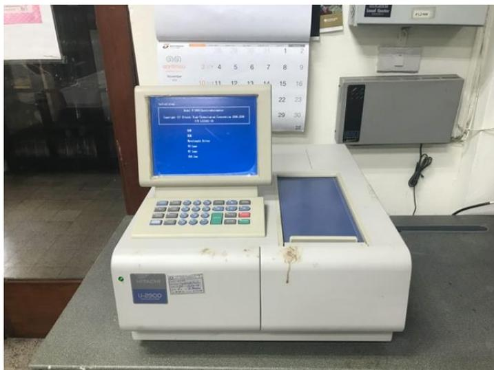
**Figure 22** A HITACHI U-2900 spectrophotometer at the Department of Mineral Resources.
