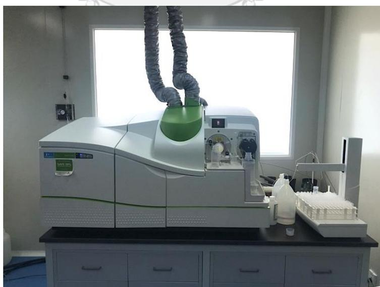
**Figure 24** A Perkin Elmer Nexion 300D ICP-MS at IEECAS.
