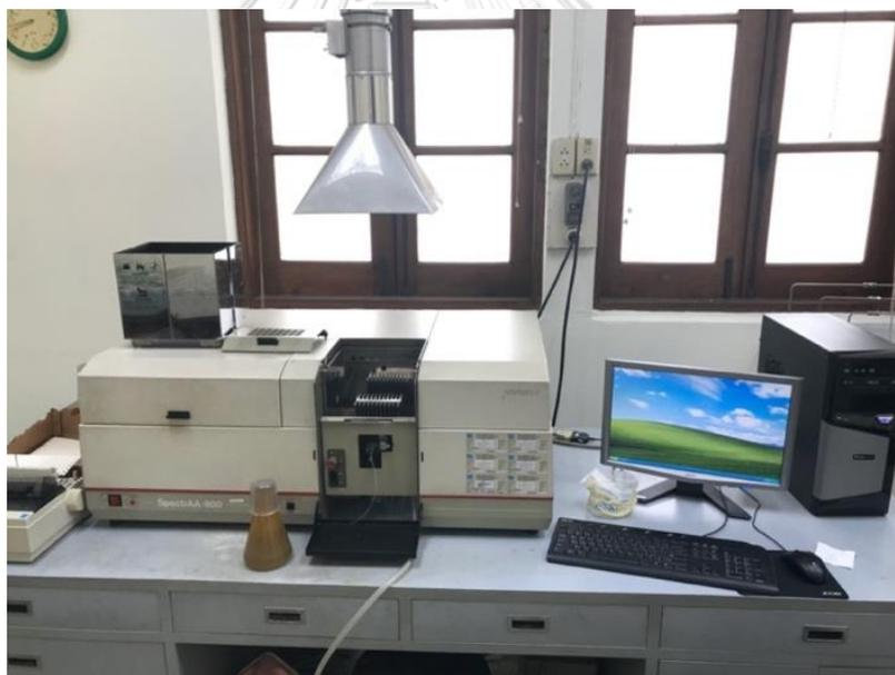
**Figure 20** Flame Furnace Atomic Absorption Spectroscopy at the Department of Mineral Resources.
