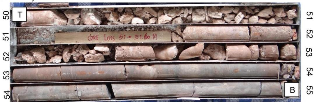
**Figure 44** Core photograph showing reddish brown mudstone until then very dark greenish gray claystone at 52.9 meters of unit C2 from K-202. T = top; B = bottom.
