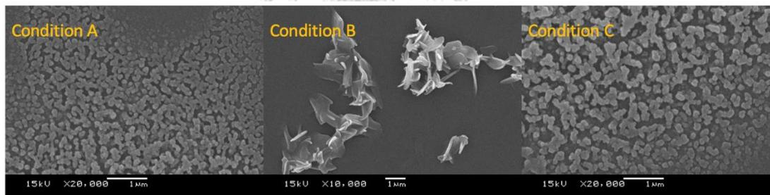
**Figure 25.** SEM of CaCit-triazine at 2, 5 and 8 hours (Condition A-C)
