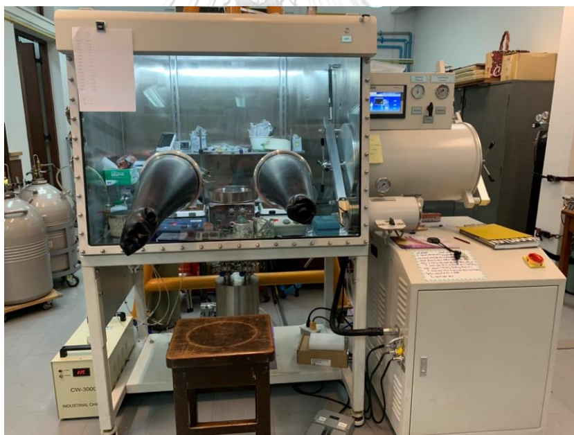
Figure 21 Photograph of the N 2 -filled glovebox (Changsha Tianchuang Powder Technology Co., Ltd.).
