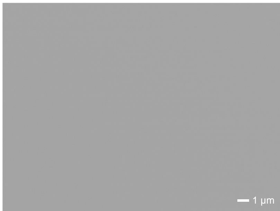
Figure 32 FESEM image shows smooth surface morphology of sputtered SnO 2 film on SLG substrate.
