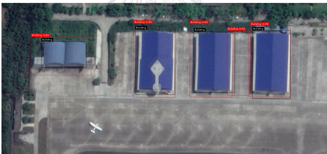
Figure 4.14: Example images of the result using the original YOLOv3 with the Jet saliency map (1378 x 643 pixels)
