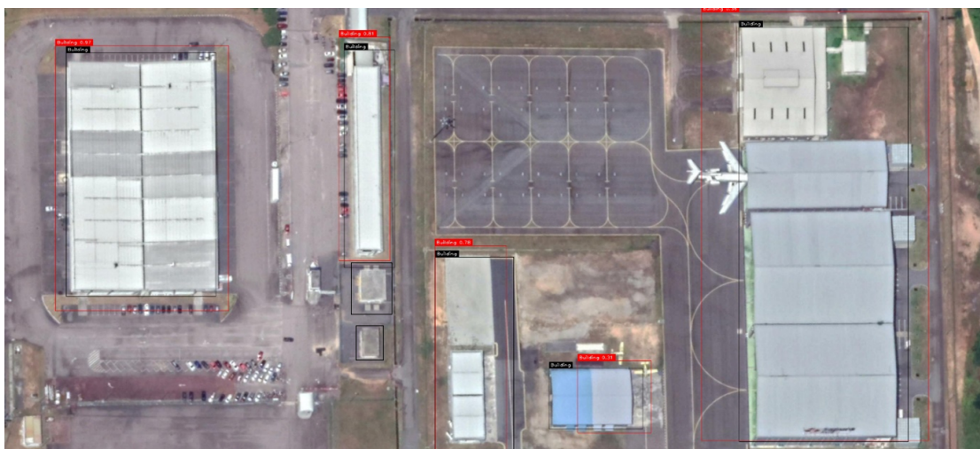
Figure 4.13: Example images of the result using the original YOLOv3 with the Jet saliency map (1377 x 623 pixels)
