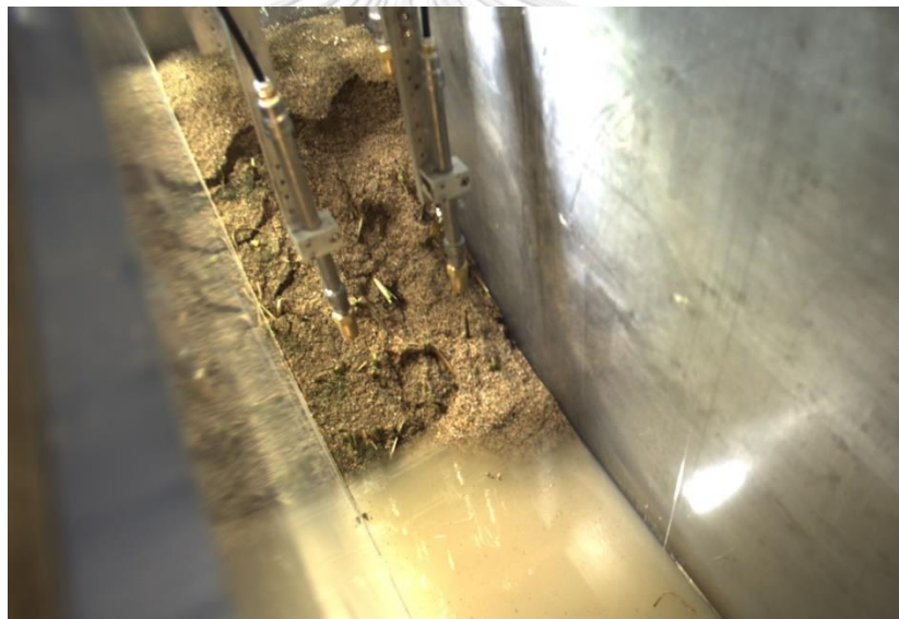
Figure 4.6 The post-test slope condition
