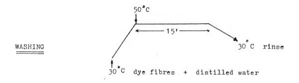
FIGURE 3.1 Schematic diagram of the dyeing and washing processes
